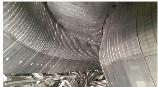
Fig. 5. The ITER-like W mono-block divertor in EAST.
