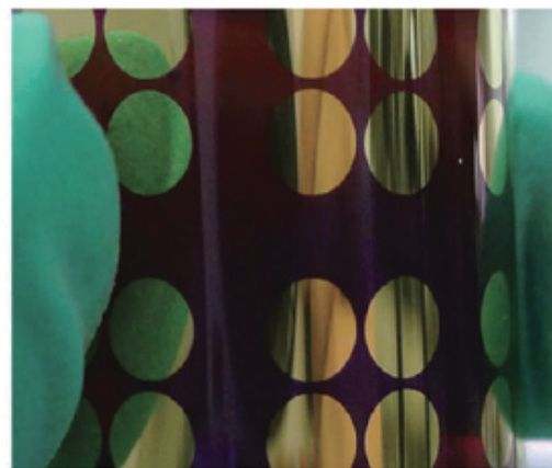
Fig. 10. Flexible perovskite solar cell with an efficiency of 15.07%.
