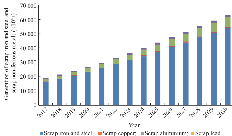
Fig. 2. Prediction of the generation of scrap iron and steel and scrap non-ferrous metals from 2017 to 2030.
