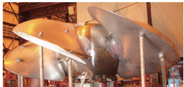
Fig. 5. Fish-friendly turbine at Wanapum power station.
