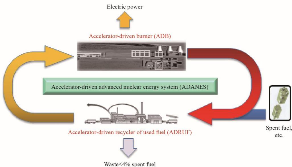
Fig. 2. Schematic diagram of the working principle of ADANES.
