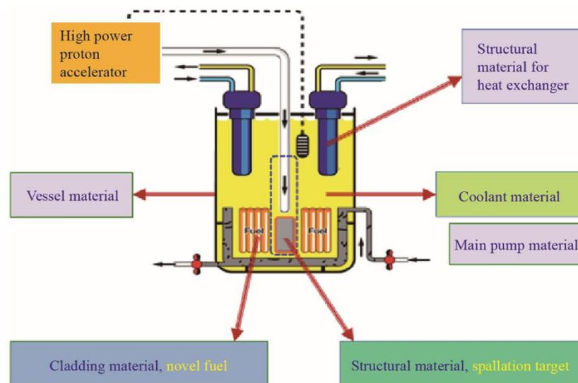
Fig. 3. Schematic diagram of material classification for different components in ADS facility.
