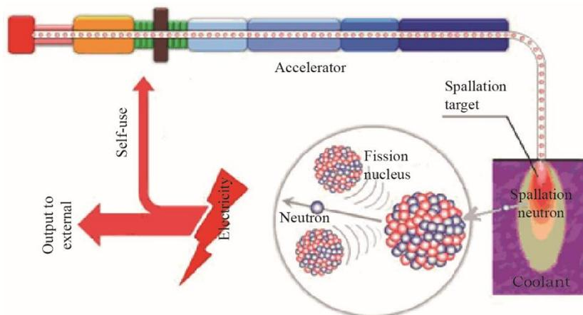
Fig. 1. Schematic diagram of the working principle of an ADS facility.
