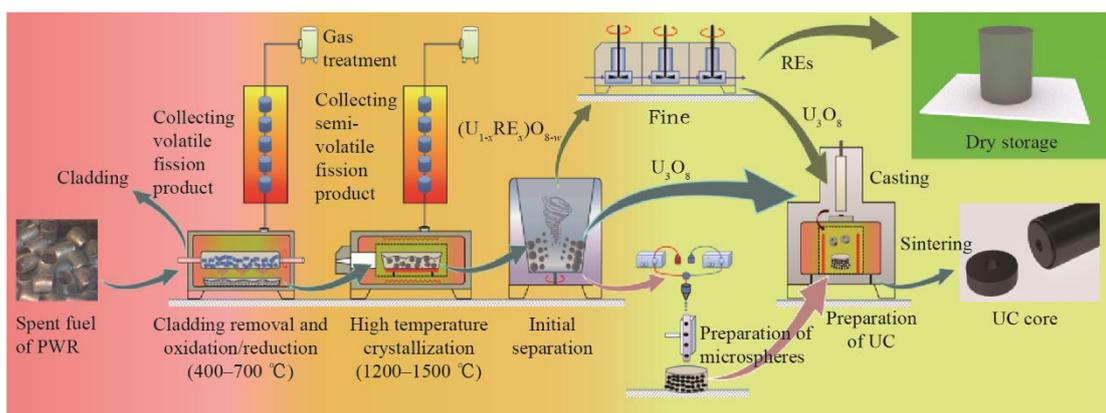
Fig. 4. Schematic diagram of the specific implementation route of the ADRUF cycle.
