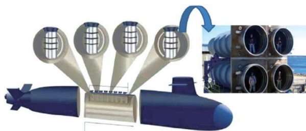
Fig. 4. Schematic diagram of common missile compartment design of a U.S. nuclear submarine.
