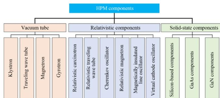
Fig. 3. Typical types of HPM components.
