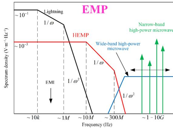
Fig. 1. Typical spectrum of different EMPs.
