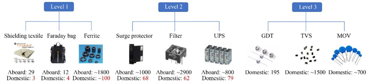
Fig. 4. Commercial products for EMP protection.
