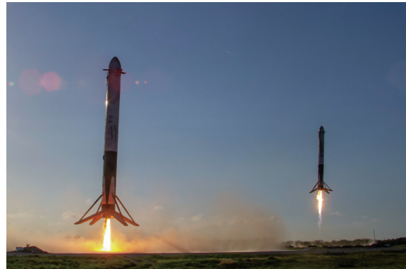
Fig. 1. The two side boosters of the Falcon Heavy touch down in Florida shortly after the rocket's launch. Credit: courtesy of SpaceX (public domain).
