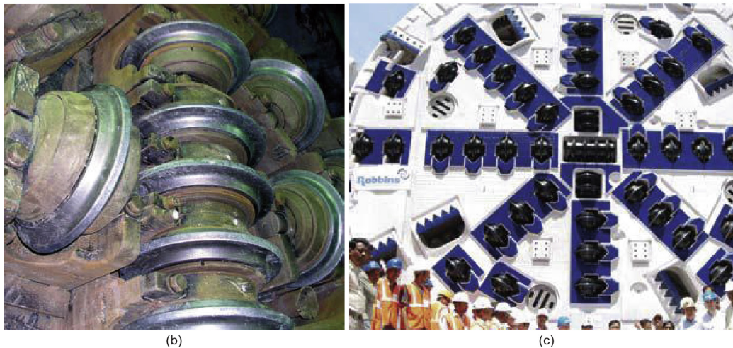
Fig. 5. (a) Schematic drawing and (b,c) pictures of the center quad (pictures from The Robbins Company).
