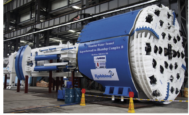
Fig. 1. A flat-profile cutterhead with back-loading cutters [22].
