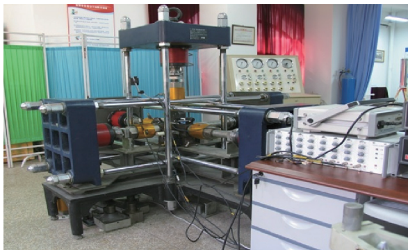
Fig. 3. Rockburst laboratory testing system.
