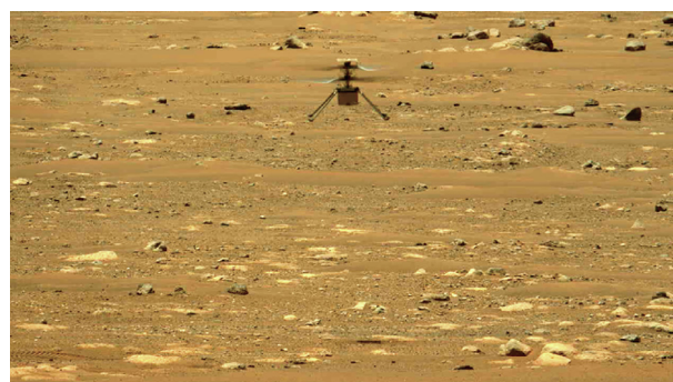
Fig. 2. The Perseverance rover snapped this photo of Ingenuity lifting off on its second flight on 22 April 2021. The copter showed more of its capabilities than on its initial flight three days earlier, traveling a total of 4 m, making three turns, and staying aloft for nearly 52 s. Credit: NASA/JPL-Caltech/ASU/MSSS.
