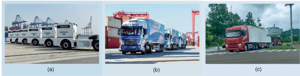
Fig. 1. Heavy-duty vehicle (HDV) platooning to collectively realize autonomous driving and efficient transportation. (a) The Westwell Q-Truck of Qomolo focuses on autonomous heavy-duty trucks for modern container logistics. (b) The 5G + level 4 (L4) project from SAIC Motor Corporation Limited (China) focuses on shortening the distance between trucks running in a queue on a bridge to improve transportation efficiency. (c) The Tongji University Guided Autonomous Logistics Vehicle Platoon (GALVP) project focuses on realizing the automatic driving of rear trucks at a low cost when the first truck is driven by a human.
