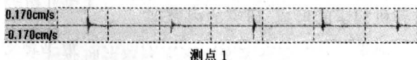
图 3 通过预裂缝传播的振速波形图 Fig.3 Waveform of vibration velocity propagated by pres-split crack
