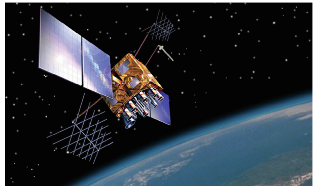
Fig. 1. Shown here in an artist's rendering, this GPS IIR-M satellite is one of a series launched between 2005 and 2009. Along with about 30 other GPS satellites in the US GPS satellite network, it circles the Earth twice daily and broadcasts time and orbit data that receivers can use to precisely determine their location. Credit: United States government (public domain).
