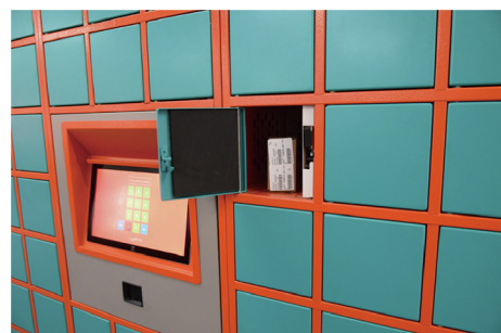
Fig. 5. The Pelebox smart locker alerts patients that their medicine is ready for collection via a text message. The system enables patients with chronic conditions to pick up their regular medicine in minutes instead of waiting hours for overstretched healthcare staff to dispense it. Credit: Technovera Pty Ltd., with permission.
