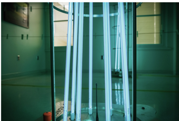
Fig. 3. The University of Nebraska Medical Center uses UV radiation to sterilize N95 masks for reuse by medical personnel [9]. Used masks are hung on clotheslines between two towers that each shine eight UVC bulbs; a 15 min exposure suffices for sterilization, and 90 masks may be treated at one time. Credit: University of Nebraska, with permission.
