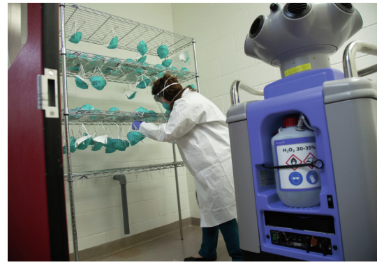
Fig. 4. Using a Bioquell (Horsham, PA, USA) hydrogen peroxide vapor generator, Duke University Hospitals staff can disinfect, for reuse, 1250 masks per cycle, and 2500 per 12 h shift [1]. A larger version of the set up manufactured and operated by Battelle (Columbus, OH, USA) can process 80 000 used masks per day, enough to supply multiple hospitals and even hospital systems [10]. Credit: Duke University, with permission.
