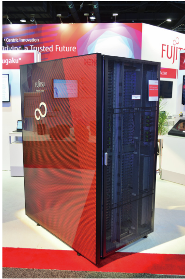
Fig. 1. One cabinet containing a set of the nearly 159 000 total nodes that coupled together power Japan's Fugaku supercomputer. The entire machine occupies 1950 m 2 , about the size of three tennis courts. Credit: Raysonho (CC BY-SA 4.0).
