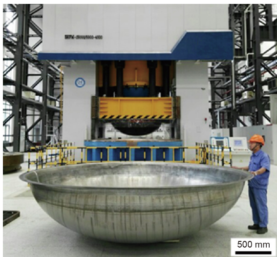
Fig. 11. Ultra-large capacity hydroforming equipment and integrated dome component. Reproduced from Ref. [36] with permission of The Japan Society for Technology of Plasticity, ©2018.
