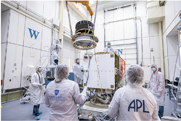
Fig. 5. Engineers position the DART's thruster assembly atop the spacecraft. Credit: NASA/Johns Hopkins Applied Physics Laboratory/Ed Whitman (public domain).
