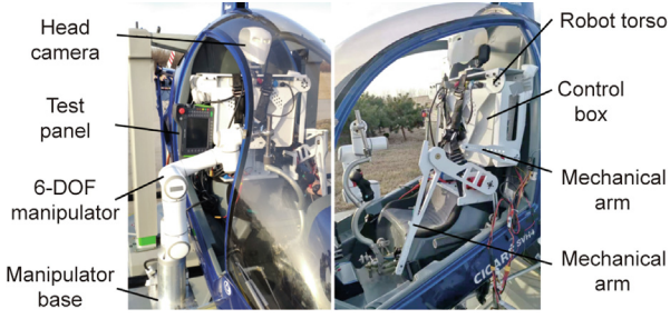
Fig. 17. Helicopter installation of the robot pilot.
