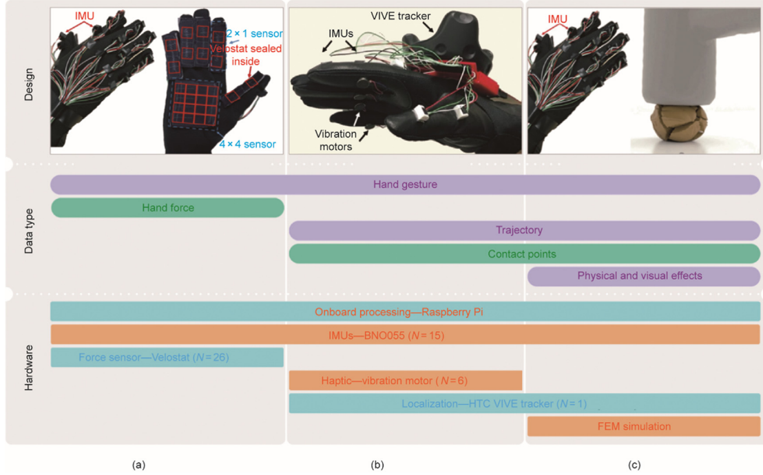
Fig. 1. Overview of our reconfigurable data glove in three operating modes, which share a unified backbone design of an IMU network that captures the hand gesture. (a) The tactile-sensing mode records the force exerted by the hand during manipulation [20]. (b) The VR mode supports stable grasping of virtual objects in VR applications and provides haptic feedback via vibration motors [23]. Contact configurations are conveniently logged. (c) The simulation mode incorporates state-of-the-art FEM simulation [19] to augment the grasp data with fine-grained changes in the object's properties. N : the number of unit(s) used in the prototype.
