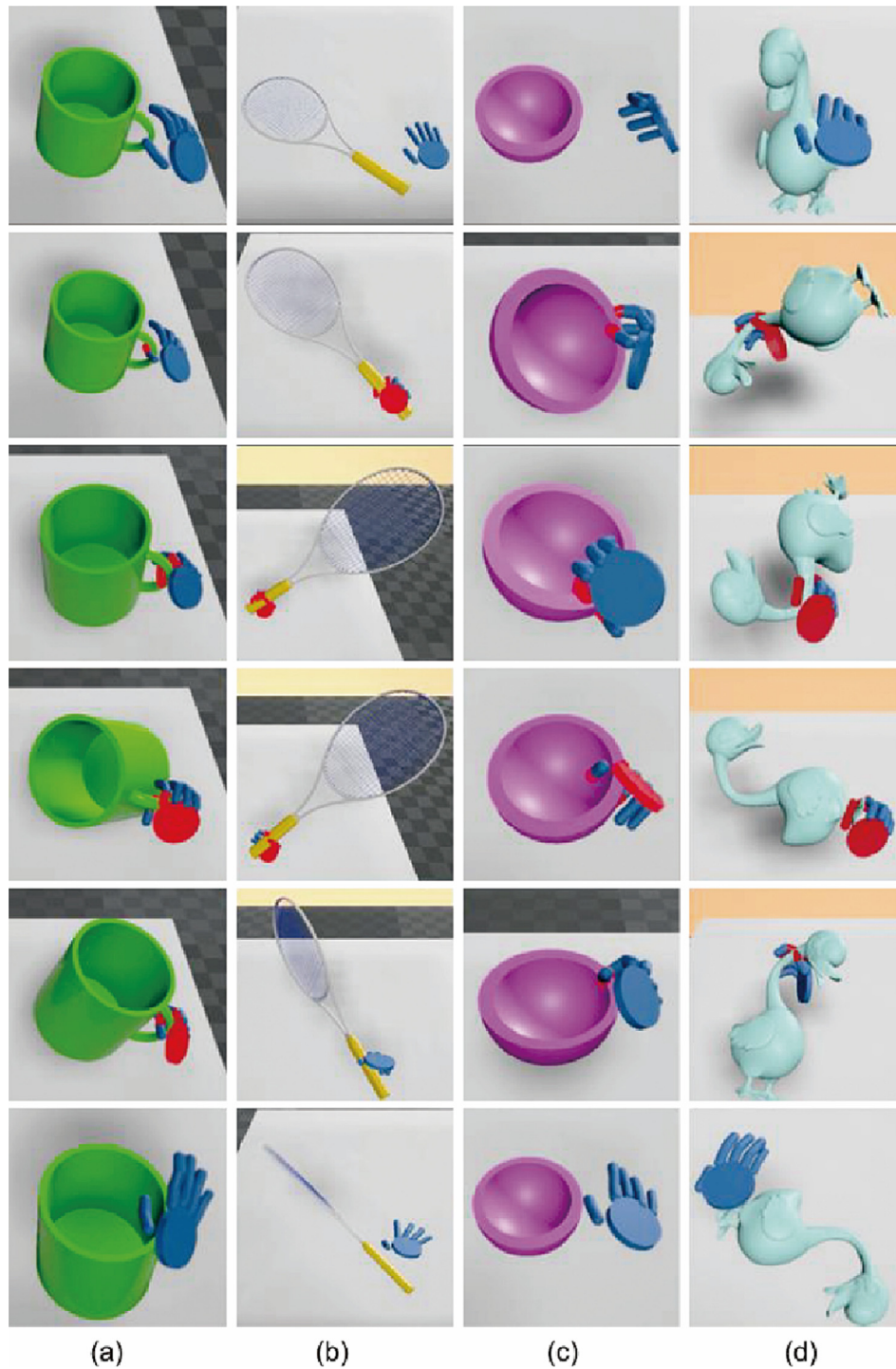
Fig. 9. Various grasp results for four virtual objects: (a) a mug, (b) a tennis racket, (c) a bowl, and (d) a goose toy. The top and bottom rows show the approach and release of the target objects, respectively. Reproduced from Ref. [23] with permission.
