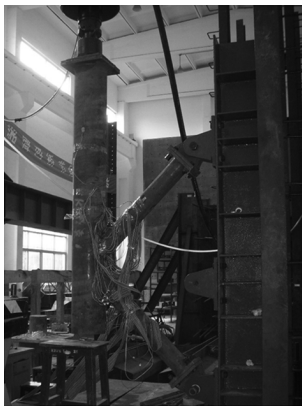
图2 K型节点试验加载装置 Fig.2 Test loading device of K joints
