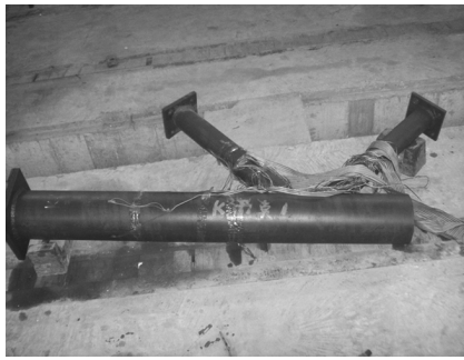
图1 平面K型钢管焊接节点试件 Fig.1 Configuration of a tubular K joints specimen
