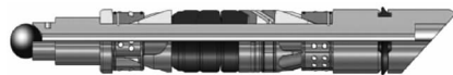
图6 Eagle Ford 快速可钻式桥塞示意图 Fig. 6 Eagle Ford fast drillable bridge plug sketch map
