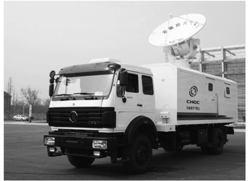
图7 新一代人工影响天气移动偏振雷达指挥系统 Fig.7 The new polarized movable radar system used in weather modification operation
