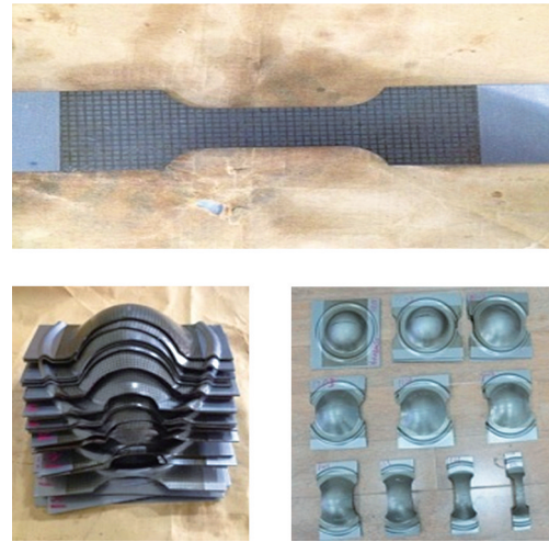
图3 试样及试验后样品照片 Fig.3 Test and tested sample
