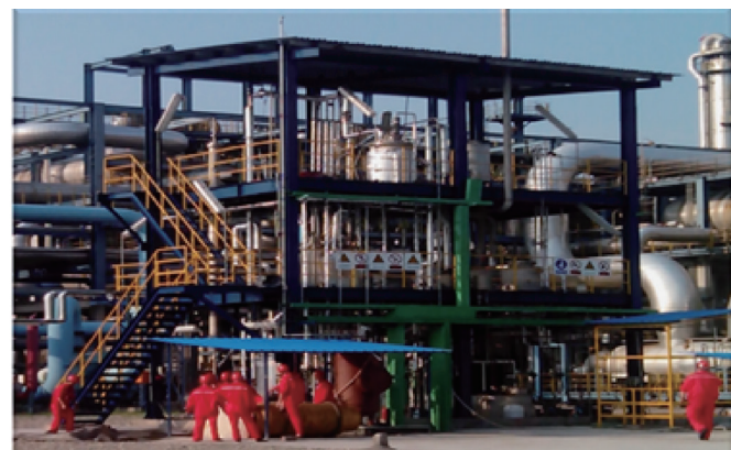
Figure 5. The pilot device at Puguang for the mineralization of flue-gas CO 2 using PG.
