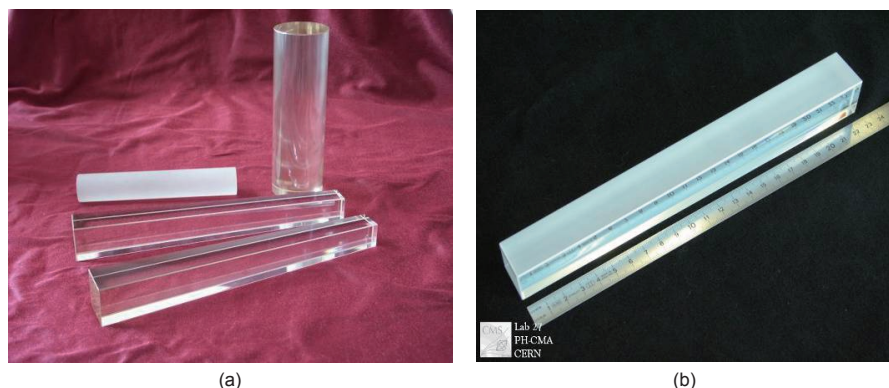
Figure 14. (a) BGO and (b) PWO crystals used in high-energy physics facilities.
