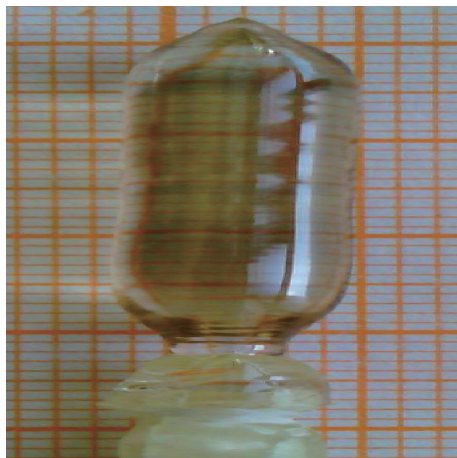
Figure 3. A Tm:Lu 2 O 3 crystal boule grown by the optical floating zone method.
