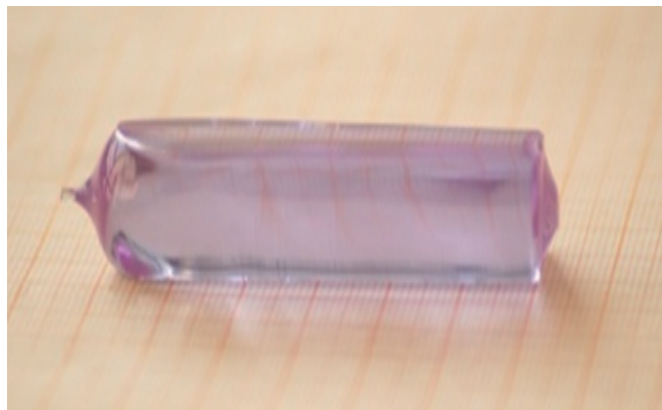
Figure 5. An 8% Nd:GdCOB crystal boule.
