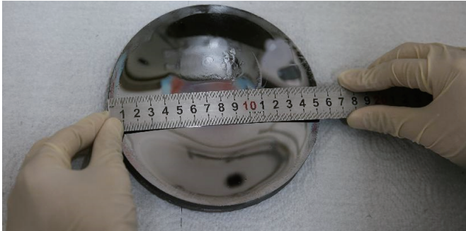
Figure 15. SiC crystal with a diameter of 6 inches (150 mm), grown by the Institute of Physics, CAS.
