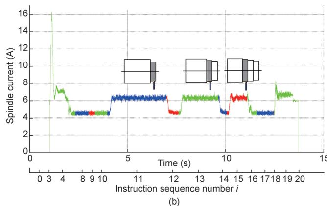
**Figure 9. A comparison of the parameters of the three-step part (a) before and (b) after optimization.**
