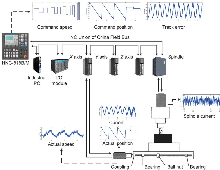
**Figure 7.** Big data acquirable inside a CNC machine tool.
