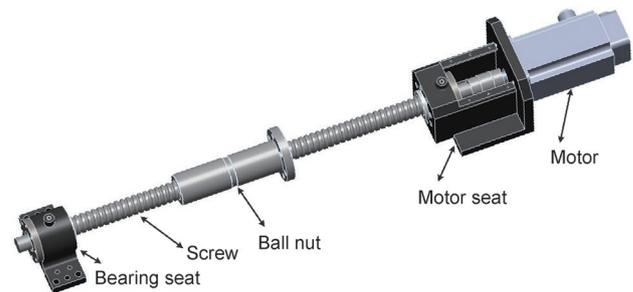
Figure 15. The feed axis mechanism of *X* axis.
