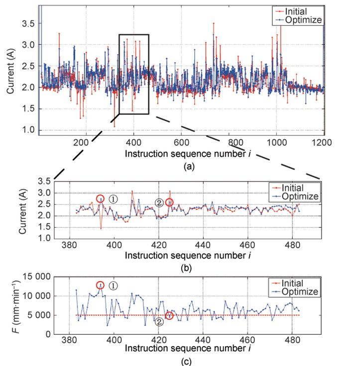
Figure 13. (a) The instruction-domain waveform of the spindle current; (b) a partially enlarged drawing of spindle current; (c) a partially enlarged drawing of feedrate.
