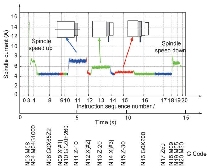
Figure 6. The current waveform of a CNC machining spindle in the instruction domain.
