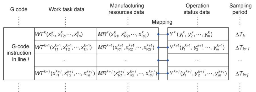
Figure 4. The mapping of work task data, manufacturing resources data, and operation status data of a CNC machine tool.
