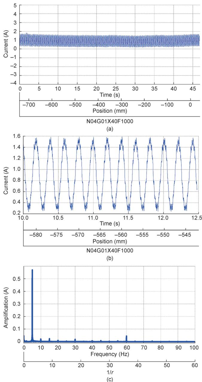
Figure 16. An analysis of the X axis current. (a) Diagram of the original current in the time domain; (b) a partial enlarged drawing; (c) the global amplitude spectrum.
