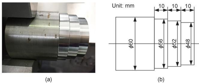
Figure 5. (a) A three-step part; (b) the dimensions.
