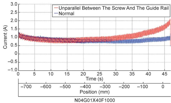
Figure 17. A comparison of the currents acquired in a normal condition (blue) and when the lead screw is not parallel to the guide rail (red).
