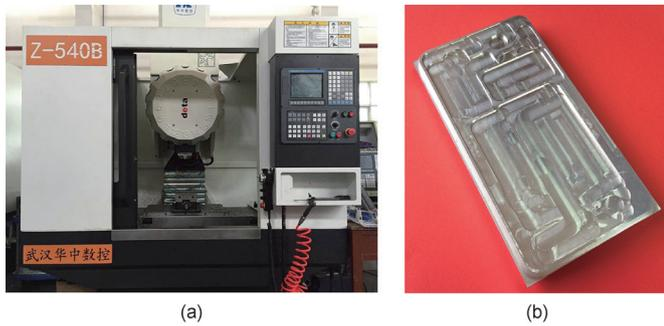
Figure 11. (a) The Z540-B drilling and tapping center; (b) the test part.
