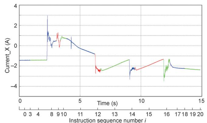
Figure 3. A waveform of the operation status data of a machine tool, using instruction domain as the horizontal coordinate.
