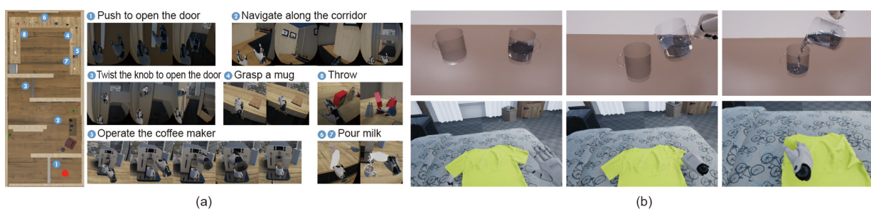
Fig. 36. VRGym, an example of a virtual environment as a large task platform. (a) Inside this platform, either a human agent or a virtual agent can perform various actions in a virtual scene and evaluate the success of task execution; (b) in addition to the rigid-body simulation, VRGym supports realistic real-time fluid and cloth simulations, leveraging state-of-the-art game engines. Reproduced from Ref. [384] with permission of Association for Computing Machinery, © 2019.
