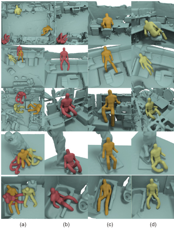
Fig. 23. (a) Top three poses in various scenes for affordance (sitting) recognition. The zoom-in shows views of the (b) best, (c) second-best, and (d) third-best choice of sitting poses. The top two rows are canonical scenarios, the middle row is a cluttered scenario, and the bottom two rows are novel scenarios that demonstrated significant generalization and transfer capability. Reproduced from Ref. [233] with permission of the authors, ©2016.
