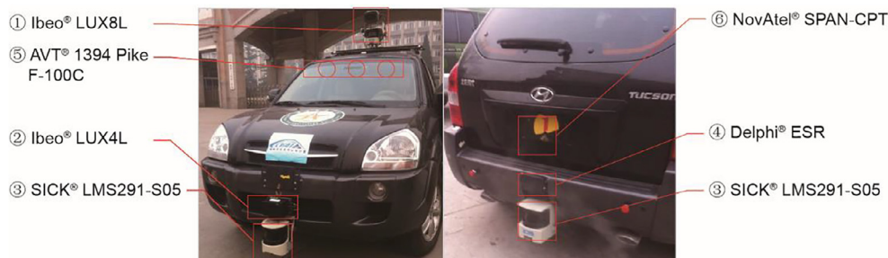
Fig. 7. Sensor deployment of the MengShi.
