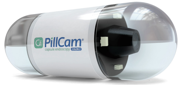
Fig. 2. The PillCam is one of many wireless endoscopy devices now available as an alternative to many conventional invasive GI procedures. The capsules contain tiny batteries and cameras that enable transmission of gut wall images to an external receiver as the device travels through the gut. Credit: Medtronic 2017.
