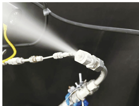
Fig. 3. The customized spray nozzle used in the MCBP field test produces a high output of very small (~50 nm dry diameter) sea salt particles by creating a high-pressure two-phase flow mixture inside a small cavity and then ejecting the air and liquid droplets in a way that avoids the immediate collision and growth of particles to larger sizes. Credit: Palo Alto Research Center, with permission.
