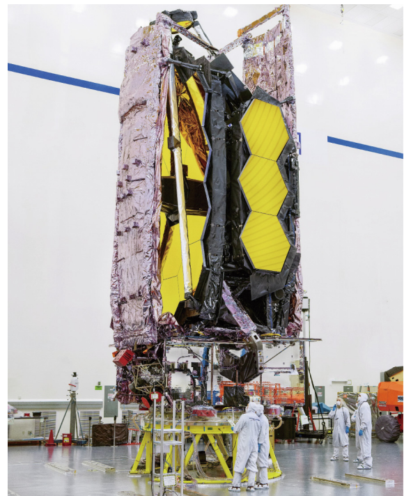
Fig. 3. Too large to fit into the fairing of a rocket, the telescope was folded into this smaller arrangement before launch. Credit: NASA/Chris Gunn (CC BY 2.0).
