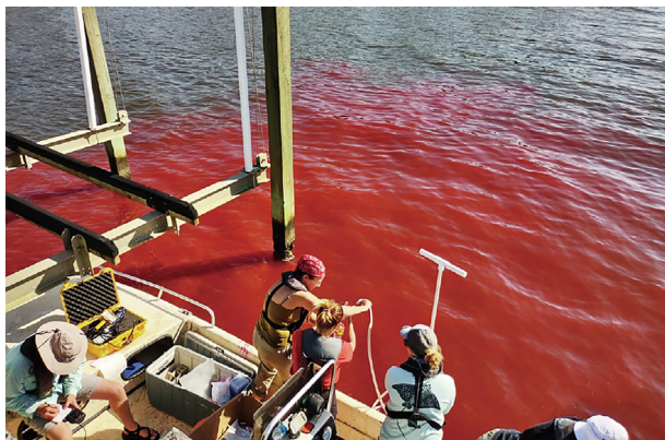
Fig. 4. In May 2022, scientists injected lime into a Florida estuary to neutralize its acidic waters and increase its absorption of CO 2 from the atmosphere. They used a red, nontoxic dye to track the movement of the lime. Credit: Wade McGillis/Ocean Acidification International Coordinating Centre (public domain).
