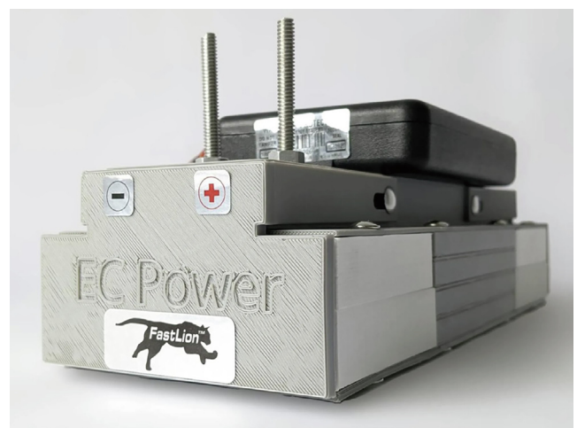
Fig. 2. The black box topping EC Power's innovative EV battery controls the 10 to 25 \mu\text{m} thick sheets of nickel foil layered within the battery that heat it from the inside out. Compared to the external thermal management systems used in most of today's EV batteries, this internal system more effectively and efficiently controls the temperature of the battery to improve its operation, including facilitating faster charging. Credit: EC Power (public domain).
