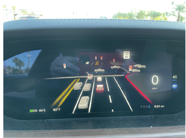
Fig. 2. Tesla Autopilot's expanded set of features, called Full Self-Driving Beta, installed in a 2022 Model S. Full Self-Driving Beta, introduced by Tesla in October 2020, includes the ability to maneuver city and residential streets, halt at stop signs and traffic lights, and make turns. Credit: Ted Drake, Flickr (CC BY-NA 2.0).
