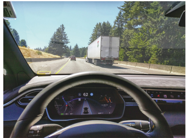
Fig. 1. Tesla's Autopilot at work controlling a 2017 Tesla Model X 75D in highway traffic. The driver-assistance system maintains a safe speed and a safe distance from the car ahead of it. Autopilot also centers the vehicle in the lane and changes lanes. Credit: Ian Maddox, English Wikipedia (CC BY-SA 4.0).
