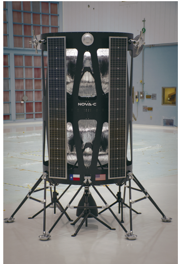
Fig. 2. The Nova-C lander from Intuitive Machines is 3 m tall, 2 m in diameter, and can tote 100 kg of cargo. The craft will carry the Lunar Vertex mission, along with three other government space agency and commercial payloads, to the Moon’s surface in 2024. The same model of lander is also booked for two previous missions scheduled to touch down near the Moon’s south pole in late 2023. Credit: NASA (CC BY 2.0).
