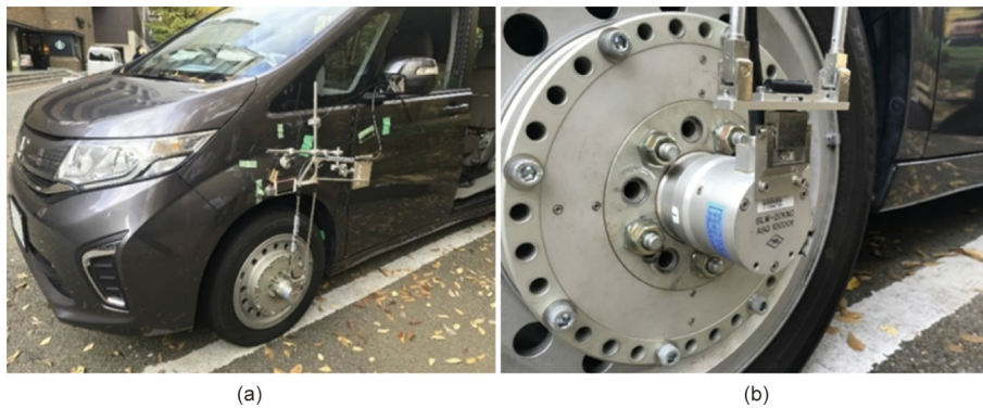
Fig. 19. Experimental setup on tire force estimation. (a) Equipped test vehicle; (b) wheel-load transducer [60].
