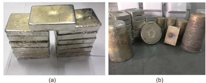
Fig. 9. Tin ingots produced by (a) microwave melting and (b) casting.
