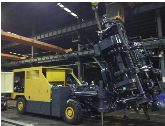
Fig. 9. Operation of the intelligent DTH drilling machine.
