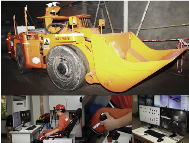
Fig. 11. An intelligent underground scraper and its remote-control platform on the surface.
