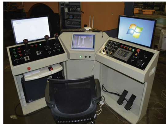
Fig. 4. Remote control platform on the surface with on-site audio and video signals.
