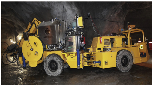
Fig. 16. An intelligent underground charging vehicle.
