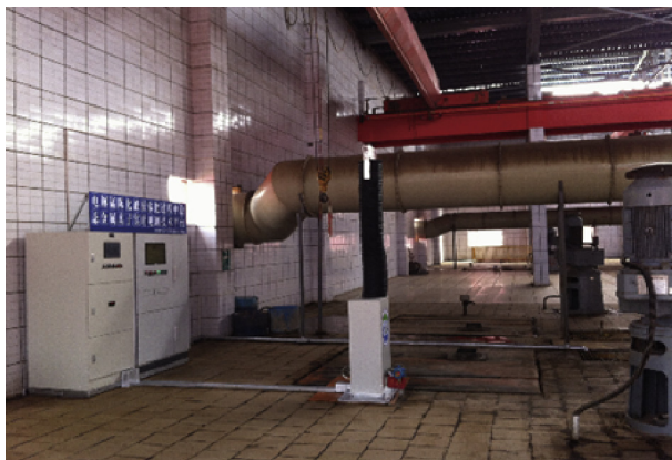
Fig. 9. Intelligent online real-time monitoring equipment for \text{Fe}^{3+} concentration in a 65\,000\text{ t}\cdot\text{a}^{-1} electrolytic manganese aging liquid colloidal process.
