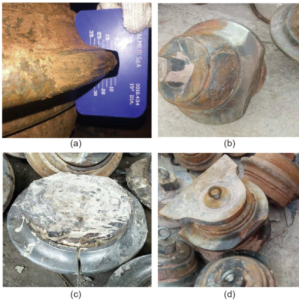
Fig. 6. Disc cutter wear. (a) Normal wear; (b) partial wear; (c) breakage wear; and (d) badly damaged.
