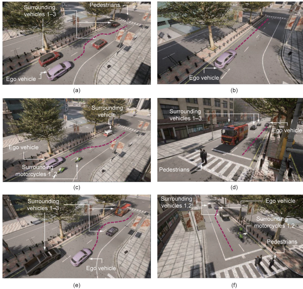
Fig. 3. Schematic diagram of the scenarios for training and testing the autonomous driving agent. (a) Scenario 0, it serves as a simple situation with all surrounding vehicles being set as stationary states. In this scenario, which was utilized only for the training stage, two pedestrians were spawned at random positions in some episodes. (b) Scenario 1, it was used to test the steady driving performance of the agent on the freeway, with the removal of all surrounding traffic participants. It was used to evaluate the anti-overfitting performance of the generated driving policy. (c–f) Scenarios 2–5, they were used to test the adaptiveness of the obtained policy in unseen situations shielded from the training stage. Moving pedestrians, motorcycles, and buses were added into the traffic scenarios. Since the interactive relationships between the ego vehicle and the traffic participants were changed, the expected trajectories of the ego vehicle were expected to differ from those in the training process. These driving conditions were set to evaluate the scene-understanding ability and the adaptiveness and robustness of the autonomous driving agent.
