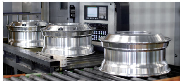
Fig. 4. Aluminum truck wheels produced via forging & flow forming by the Shandong Meika Wheel Co., Ltd.
