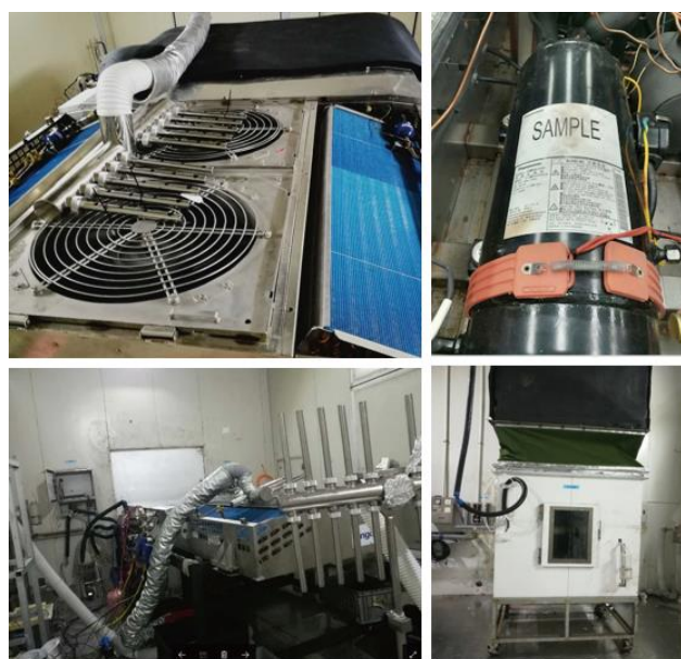
Fig. 11. Low-temperature air source heat pump prototype and testing device for electric bus.
