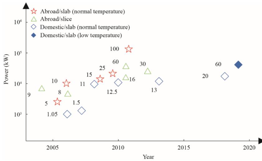
Fig. 2. Development of single-caliber solid-state lasers with block structure represented by slab and slice.
