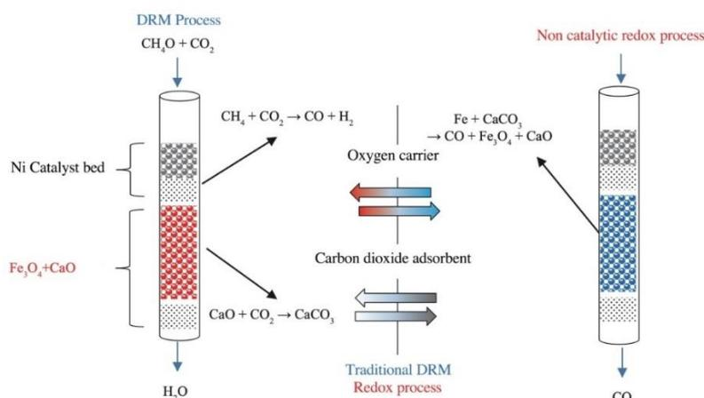
Fig. 2. DRM and high temperature oxidation–reduction process.
