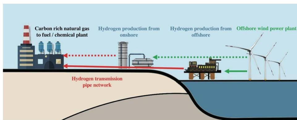
Fig. 4. Offshore wind power hydrogen production and CO<sub>2</sub> Chemical utilization technology route.
