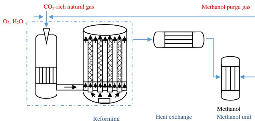
Fig. 3. Process flow diagram of the integrated technology of methanol production from CO<sub>2</sub>-rich natural gas.
