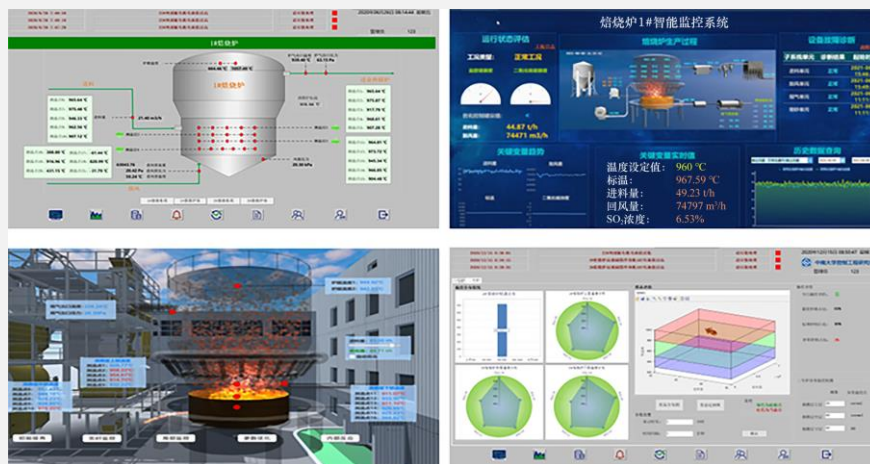
Fig. 8. Intelligent monitoring solution for zinc roasting furnace.
