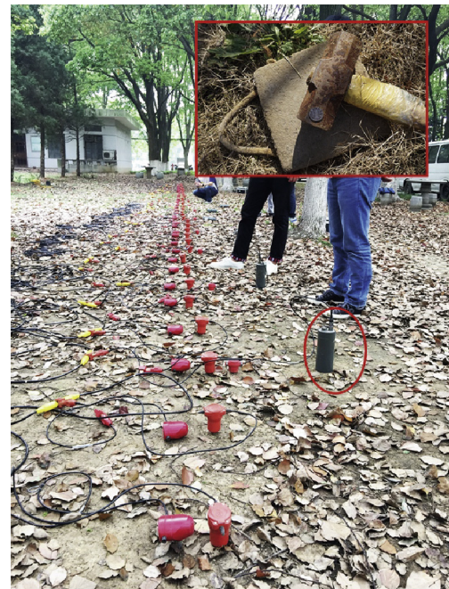
Fig. 2. Combined active-passive surface-wave experiment in the backyard of the Institute of Geophysics and Geomatics.
