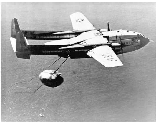
Fig. 2. In August 1960, a US Air Force plane attempts a bucket catch to retrieve the film capsule released by a Corona satellite. The capsule hangs just below the parachute the plane is about to capture. Credit: US Air Force (Wikimedia, public domain).
